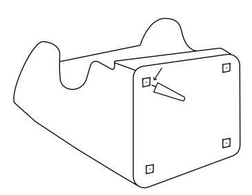
20 screws of 5x50 mm are fixed to the four corners of the berber together with the leg with the help of a drill.
