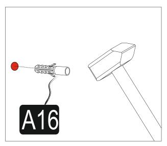
Attach the plugs to the drilled places.
