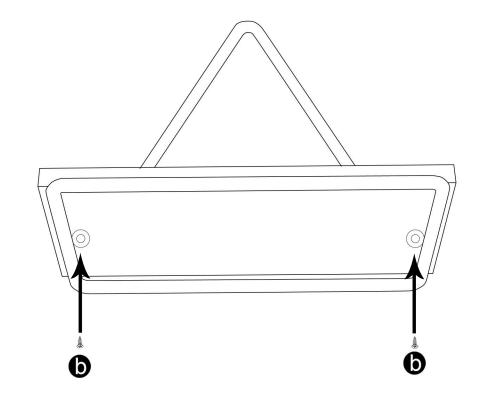
Screw the wooden shelves into the screw slots on the wire.
