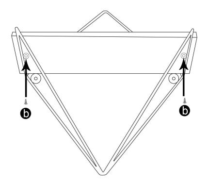
Screw the wooden shelves into the screw slots on the wire.
