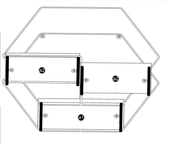
Hang the rack you prepared into the wall dowels by screwing.
