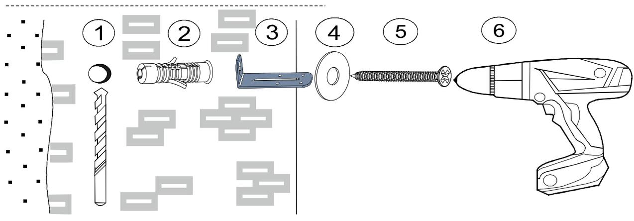
Check the wall type before installation of dowel. Wall is drilled with equal diameter of dowel. [08mm] Universal Plastic Dowel provides the general purpose usage. Requires two stages assembly. Dowel can be different type according to the wall type. [E.g. Plaster sheet partition wall, gas concrete, hollow brick wall]. If required, use appropriate dowels and screws.
