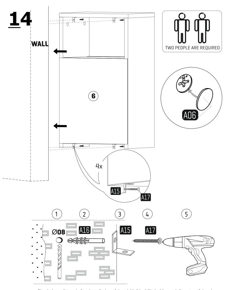
Check the wall type before installation of dowel. Wall is drilled with equal diameter of dowel. **[08mm]** Universal Plastic Dowel provides the general purpose usage. Requires two stages assembly. Dowel can be different type according to the wall type.
