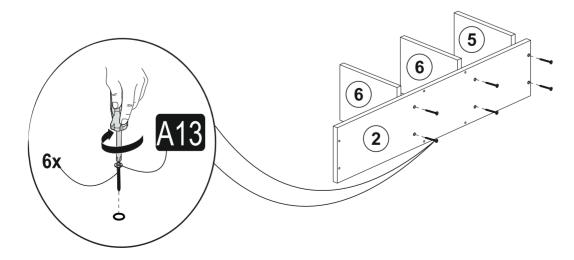
**step g**\*Please attach **the part we installed in step f** as shown below
